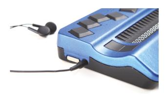
Up to four devices can be connected simultaneously to the Actilino: up to three Bluetooth devices and one USB.
